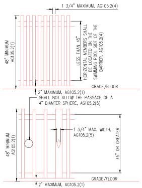
5. Where the barrier is composed of horizontal and vertical members and the distance between the tops of the horizontal members is 45 inches or more, spacing between vertical members shall not allow passage of a 4 inch diameter sphere. Where
