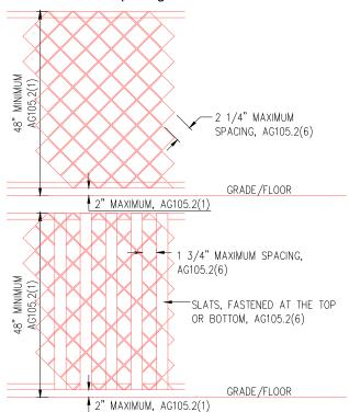
7. Where the barrier is composed of diagonal members, such as a lattice fence, the maximum opening formed by the diagonal members shall not be more than 1 3/4 inches.
