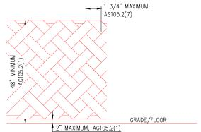
8. Access gates shall comply with the requirements of Section AG105.2, Items 1 through 7, and shall be equipped to accommodate a locking device. Pedestrian access gates shall open outward away from the pool and shall be self-closing and have a self-latching device. Gates other than pedestrian access gates shall have a self-latching device. Where the release mechanism of the self-latching device is located less than 54 inches from the bottom of the gate, the release mechanism and
