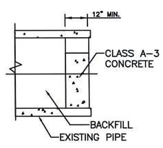
SECTION OF CONCRETE PIPE PLUG
