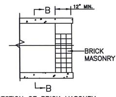
SECTION OF BRICK MASONRY PIPE PLUG
