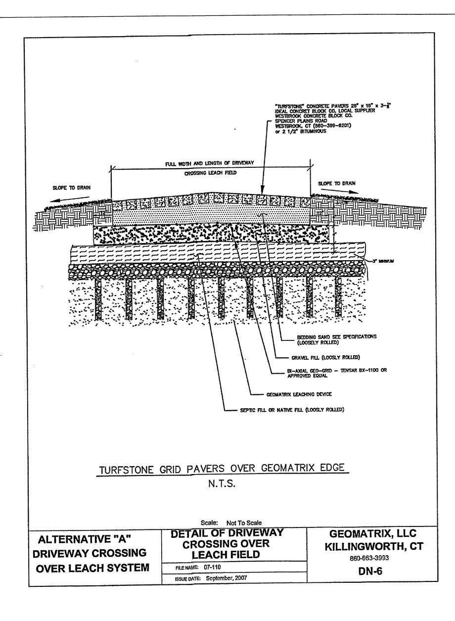
Geomatrix GSTTM Leaching System **Installation Instructions** This installation procedure serves as a general overview of the installation procedure for Geomatrix GST. The system drawings should be strictly adhered to and an authorized representative of Geomatrix Systems, LLC must be present unless the contractor is certified by Geomatrix Systems. 2. Prepare site and remove any trees with a drip line falling within 10 feet of the leaching system.
