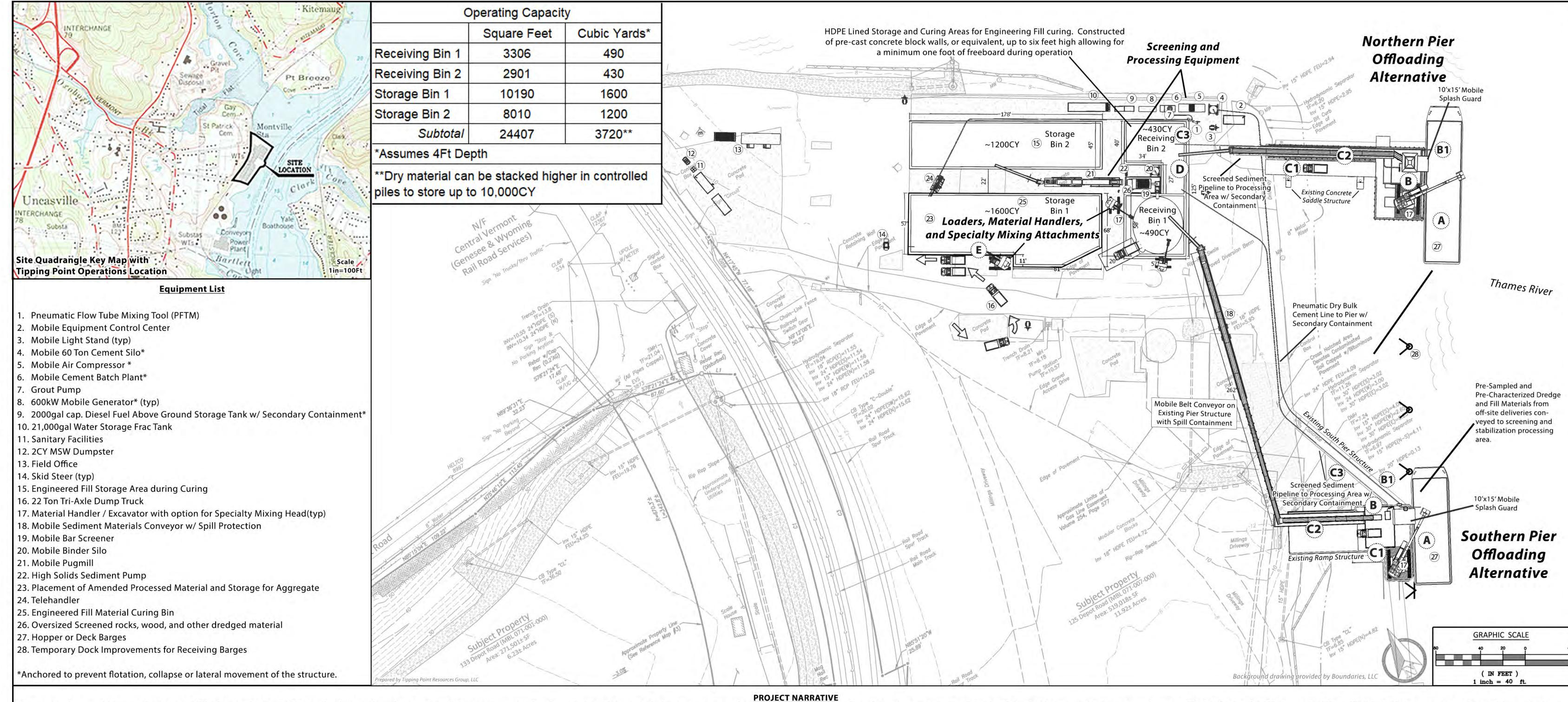
The proposed project/site operations consist of the intended use of 125 Depot Road for receiving large rock and other construction related aggregate which may include sediment processing to produce engineered fill products from sediments stabilized with Portland cement. Subsequent transloading will take place at the 125 Depot Road that will include offsite transport to the receiving entity. Conversely, water-borne scows may receive construction material for over the water transport.
