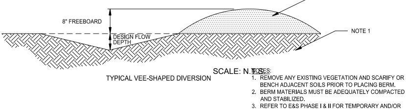
4. BERM SHALL NOT BE CONSTRUCTED OF TOPSOIL. **DIVERSION BERM DETAIL**
