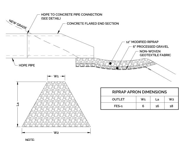
IN ACCORDANCE WITH CT DOT DRAINAGE MANUAL SECTION 11.13 - OUTLET PROTECTION, ALL APRON STONE SHALL BE INTERMEDIATE RIPRAP (DISCHARGE VELOCITY 8-10 FT/S) **RIPRAP APRON** NOT TO SCALE
